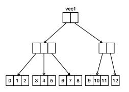
The indexing operation is **effectively constant time** because the depth of the tree is **logarithmic** in the number of elements.
