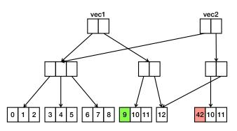
The update operation is also **effectively constant time** because the depth of the tree is **logarithmic** in the number of elements.
